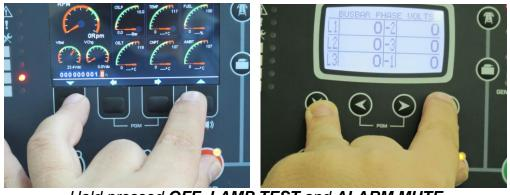
Hold pressed OFF, LAMP TEST and ALARM MUTE
