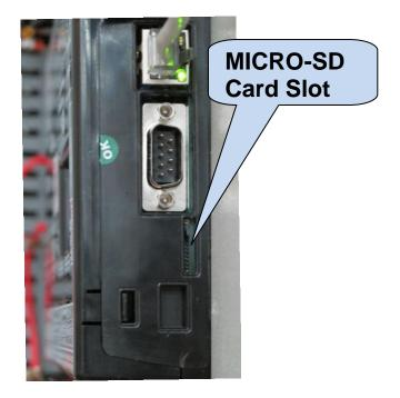
The micro-SD card slot is available in units with COMM option. The slot is of push-in push-out type. When pushed in, the card is firmly held by its connector.
