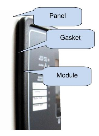
The rubber gasket provides a watertight means of mounting the module to the genset panel. Together with the gasket, IEC 60529-IP65 protection can be reached from the front panel. A short definition of IP protection levels is given below.
