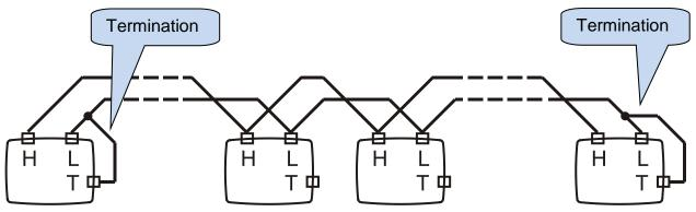
Figure illustrating the Datalink termination from two ends
