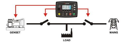
The **Export to Mains** mode allows the multi genset system to supply the mains power grid under constant power factor. Thus the multi genset system will be part of the mains power supply system.
