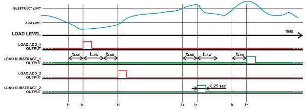
t1: the load goes below the Multi Load Add Power Level.
