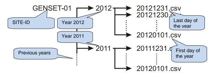
The unit will record data in a directory named with the first 11 characters of its site-id parameter. In order to avoid confusion between records, it is highly recommended to configure the site-id parameter accordingly to the genset installation place. Thus the same memory module may be used for recording in different controllers,
