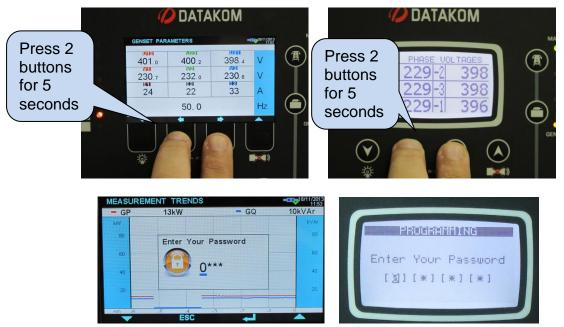
Skip the password entry screen by pressing the button 4 times. The screen below left will come.
