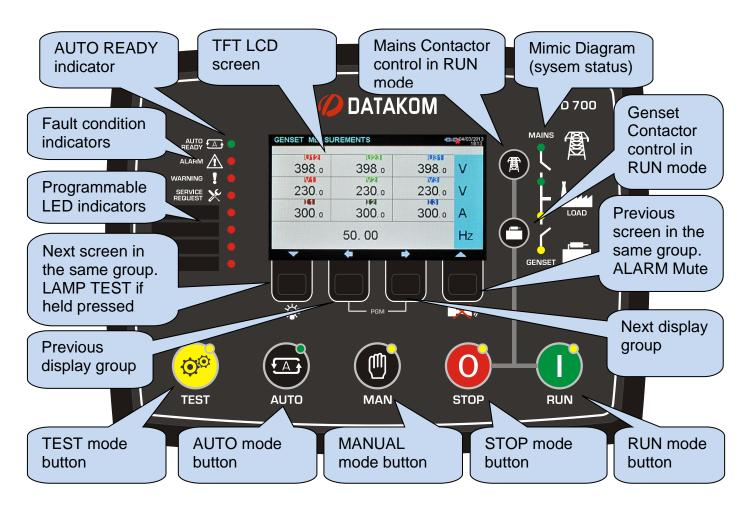
When the engine hours <u>OR</u> the time limit is over, the **SERVICE REQUEST** led (red) will start to flash and the service request output function will be active. The service request can also create a fault condition of any level following parameter setting.
