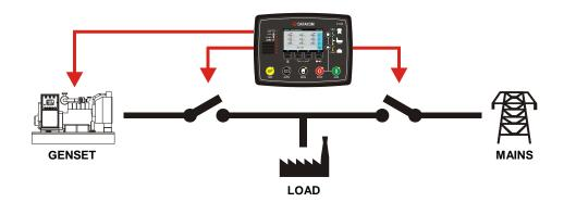
When AMF functionality is selected, there are a number of adjustable parameters causing parallel operation to the grid:
