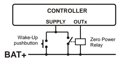
The controller wakes-up on applying the power through the "wake-up" pushbutton. Then it will immediately activate the zero power output which will cause the zero power relay to feed the controller.
