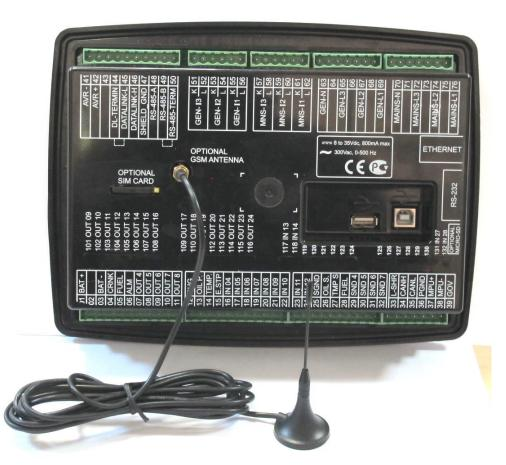
The module requires a GPRS enabled SIM card for full functionality. Voice-only type SIM cards will usually not function properly.
