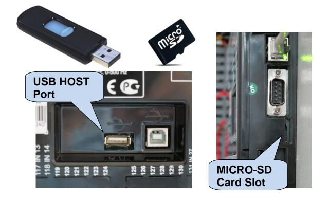
The USB-Host port and MICRO-SD card slot are available with COMM option.
