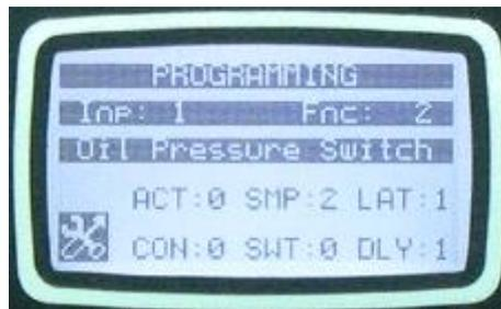
The unit has 8 digital inputs. By using external input extension modules, up to 40 inputs in total are available.
