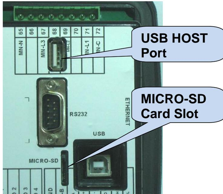
The micro-SD card slot is available in units with COMM option. The slot is of push-in push-out type. When pushed in, the card is firmly held by its connector.
