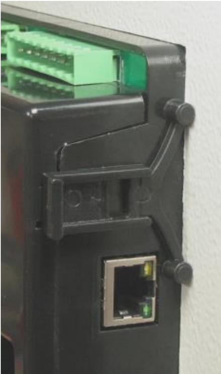
Installation of self retaining type bracket
