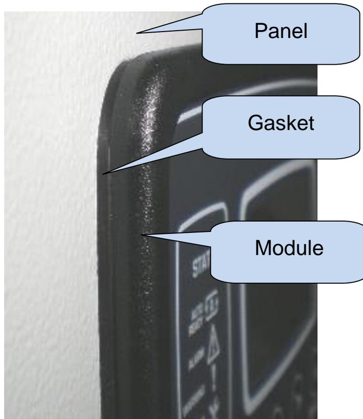
The rubber gasket provides a watertight means of mounting the module to the gasket panel. Together with the gasket, IEC 60529-IP65 protection can be reached from the front panel. A short definition of IP protection levels is given below.
