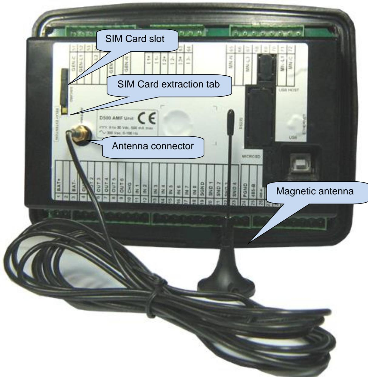
The module requires a GPRS enabled SIM card for full functionality. Voice-only type SIM cards will usually not function properly.
