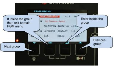
Navigation inside a group is made also with ▼and ▲ buttons. A list of available parameters will be displayed. Selected parameter is shown in reverse video (blue on white). In order display/change the value of this parameter, please press MENU▶button.
