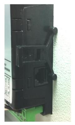
Installation of self retaining type bracket
