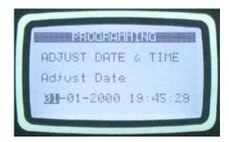
These parameters allow adjusting the battery backup real time clock of the module. Once set, the clock will continue to run even if DC power is removed from the unit.
