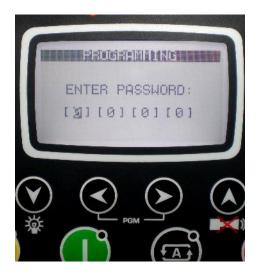
Skip the password entry screen by pressing the button 4 times. The screen below left will come.
