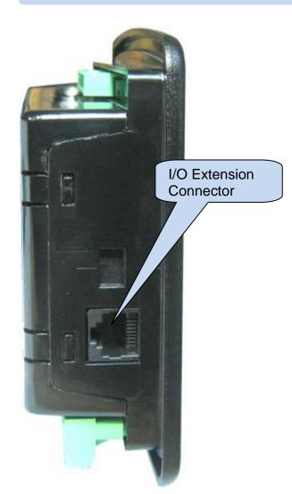
The module provides resources for 16 additional digital inputs and 16 additional digital outputs.
