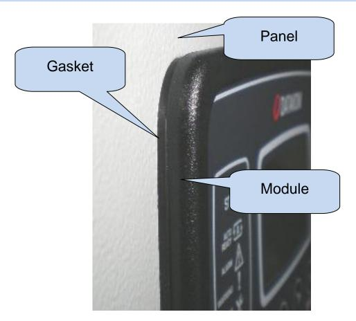
The rubber gasket provides a watertight means of mounting the module to the genset panel. Together with the gasket, IEC 60529-IP65 protection can be reached from the front panel. A short definition of IP protection levels is given below.
