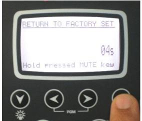
Hold pressed OFF, LAMP TEST and ALARM MUTE Hold pressed ALARM MUTE
