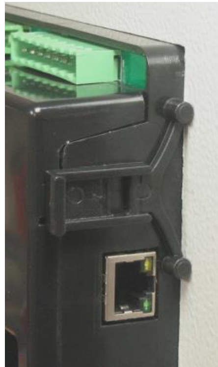
Installation of self retaining type bracket
