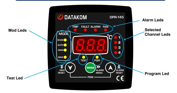
**SELECTED CHANNEL LEDS:** indicates the related channel to alarm or information on display.
