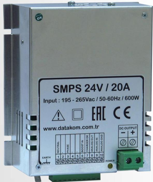
The charger measures internally its output current and provides a 0-10V analog output. This signal may directly drive measurement units.
