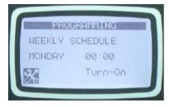
In some applications, it is desired that the compressor activates automatically only during office hours. The weekly schedule allows for these types of applications.
