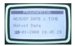
Date-time info is received from the battery supported real time clock in the controller.
