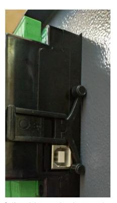
Self-retaining type bracket mounting
